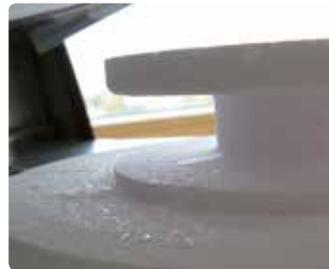
Check the sinter tray on a regular basis to see if it is free of dust and free it from dust if necessary. Contact reactions at high temperatures may lead to damage of the zirconium oxide surface. They can be detected as white spots, for example.
