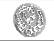
CAD/CAM-manufactured framework (CNC milling)
