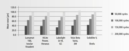
Wear resistance of SR Nexco tested according to the ACTA method in approved polymerization units
