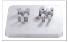
CAD/CAM-manufactured framework (selective laser sintering)
