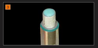
Seal screw channel with wax
